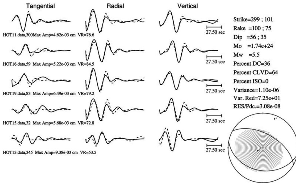
**Figure 3.** Three component observed and synthetic displacement seismograms for a point-source moment tensor inversion for another, independent set of stations, whose locations are shown in Figure 1. Compare with Figure 2a.
