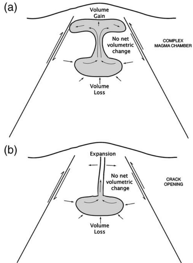
**Figure 6.** Sketch of tested models with two compensating sources reproducing a vertically oriented CLVD in dilatation (where volumetric exchange is equal and opposite in sign): (a) a complex magma chamber and (b) an implosive source and a vertical, horizontally opening crack above.
