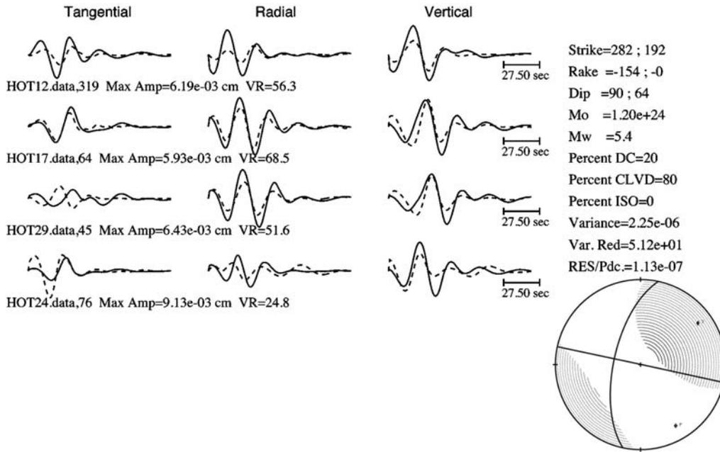
**Figure 5.** The inversion results for a point-source moment tensor inversion for the case of poor azimuthal coverage. HOT01 and HOT22 are excluded from the inversion, and this results in a strong horizontal CLVD. Compare with Figures 2a and 3.
